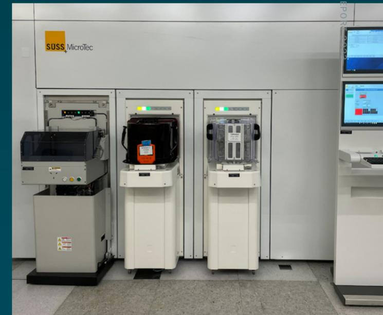
**Suss MicroTec's 200/300 mm automated tool for debonding 2D materials (TMDCs) from a growth wafer. Credit: SUSS MicroTec Solutions GMBH & CO KG**
