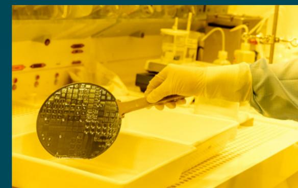
**Above:** The first step in the fabrication process is the wafer coating and development. Credit: AMO
