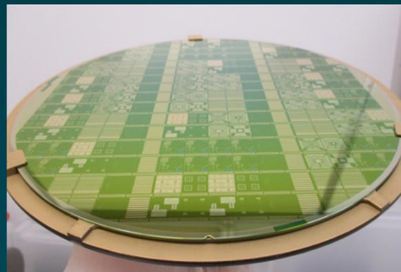
A graphene-integrated wafer.
